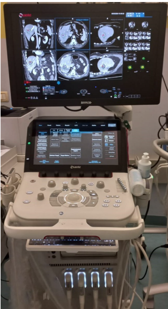
Figure 4 Augmented Ablation Suite. Pre-ablation and post-ablation computed tomography datasets are displayed on the monitor of the ultrasound machine.
